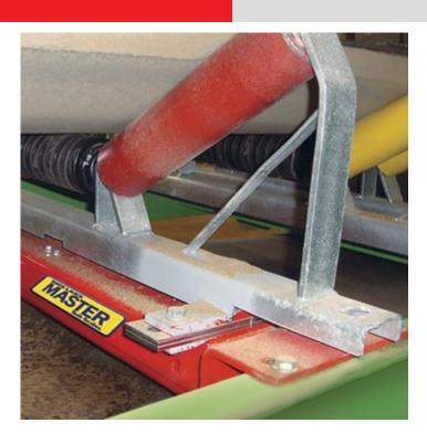
The BS311 MASTER belt scale weigh frame is suitable for medium to heavy capacity belt conveyors. Easy to install and in standard or custom made dimensions, it easily fits on the conveyor frame by using only four bolts.
